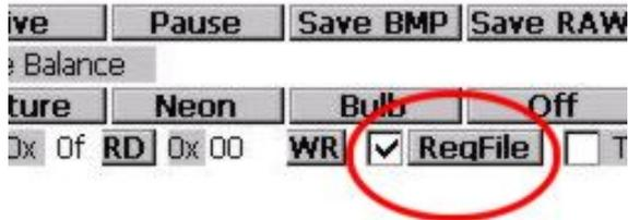
To make this settings permanent, call the *savereg* function after closing the demo application. By this, the contents of the register file will be uploaded to the camera automatically every time the demo application is started.
